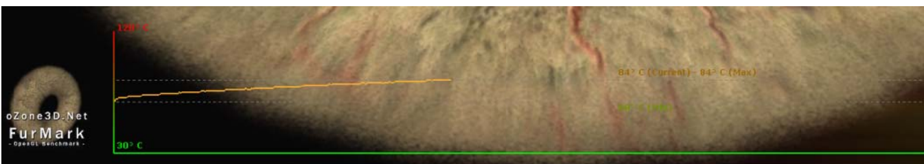
FurMark Full load of N520-053-Q01: Max Temperature 84°C
