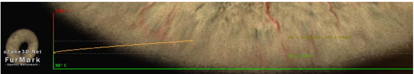
FurMark Full load of N520-203-Q01: Max Temperature 75°C
